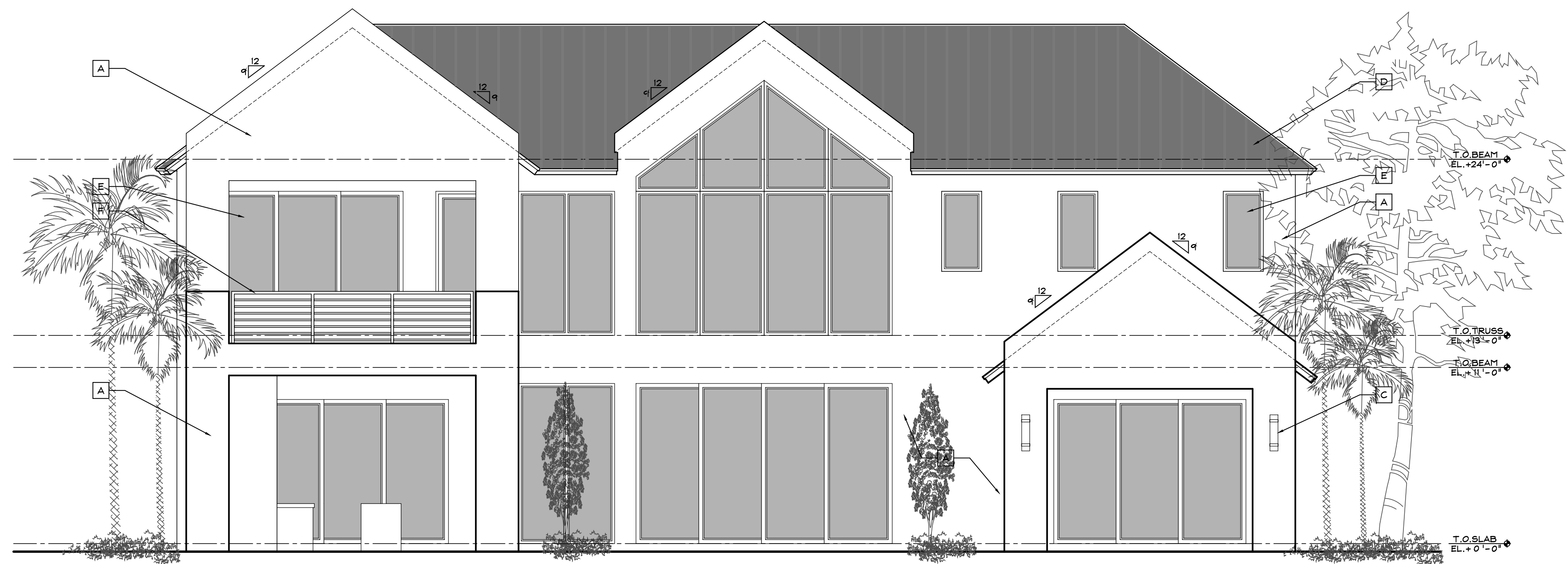
Proposed South Elevation
